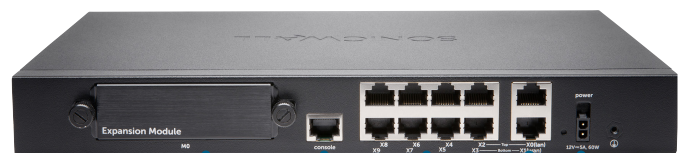
Expansion module Slot (future) Console port 8x1GbE switch (configurable) X0 LAN Port X1 WAN Port Secure power
