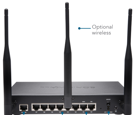
Console port 6x1GbE switch (configurable) X0 LAN Port X1 WAN Port Secure power
