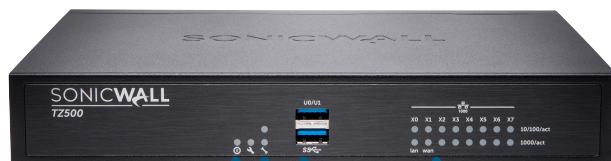
Power LED Test LED USB port (3G/4G WAN Failover) Link and activity Indicator LEDs
